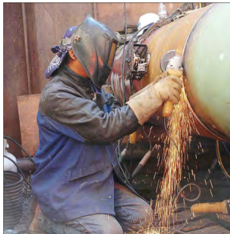
Smoothing out the inside weld in preparation for the outside weld.
