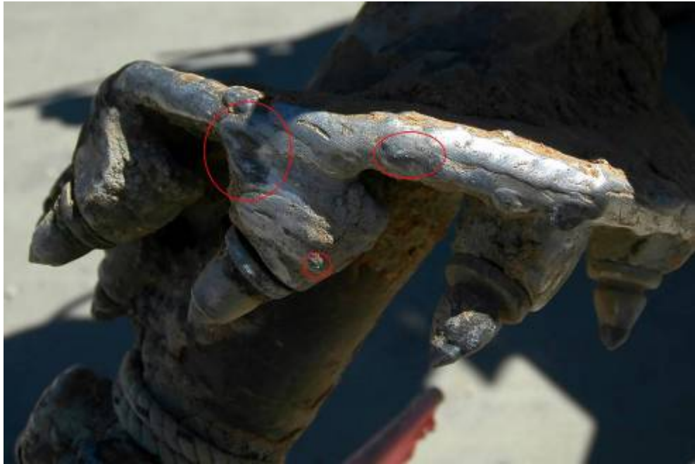
Arcing Marks Found on Auger – Approximately 29” from Ground:
