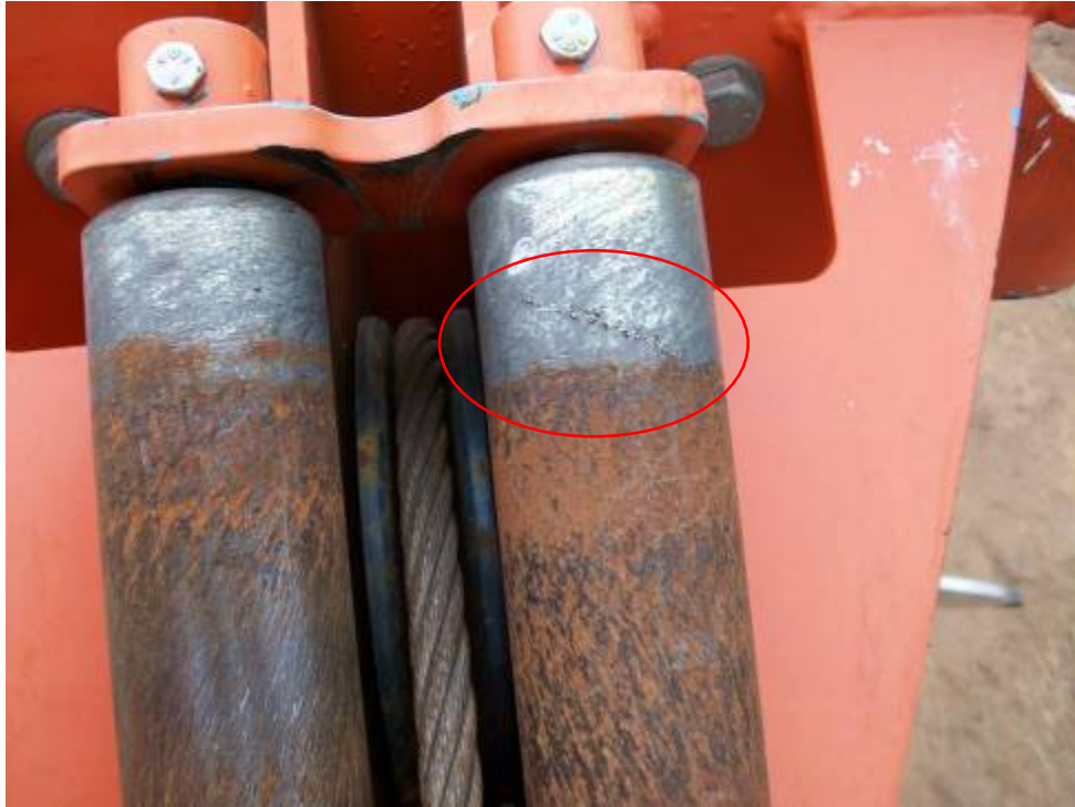
Arcing Marks Found on Auger – Approximately 29” from Ground:
