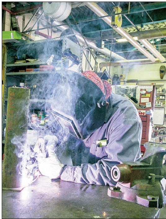
Right: Welder/Mechanic Bronc Cutler repairs a section of pipe on the unit #1 hydrogen cooling water system.
