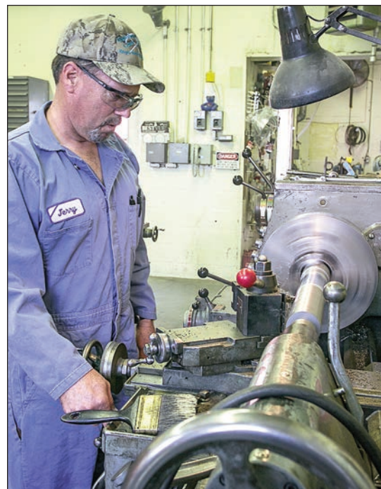
Left: Machinist Jerry Espinoza builds a new shaft for the unit #1 hydrogen cooling water pump.
