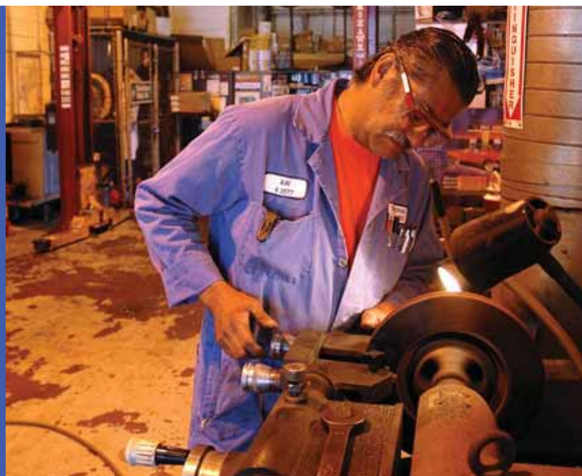
Turning rotors in the bus shop is Gasoline Propane Mechanic Raymond Lucero.
