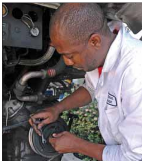
BELOW: Eric Okungbowa, "A" Mechanic Trainee, changes broken pulley on an AC compressor.
